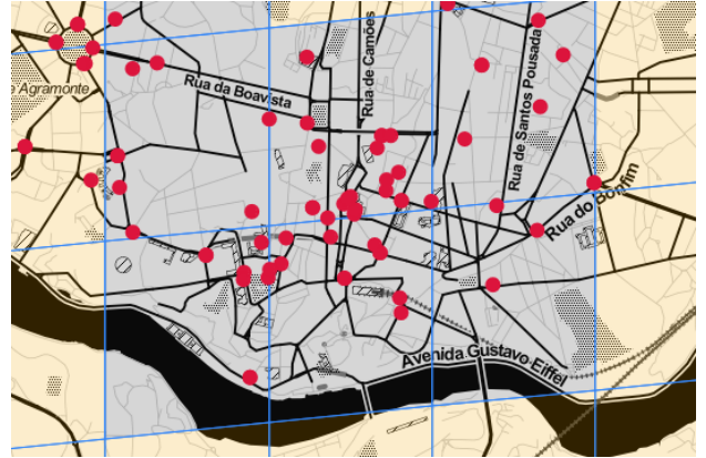
Fig. 1: city centre of Porto with RSUs and S2 Cells. Created using leaflet[2]
